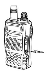
A discharged battery will require between 6-10 hours to fully charge via the AC-to-DC Adapter. While the DX15 can be used to receive and/or transmit while charging, such usage will increase the time it takes for the battery to fully charge.
