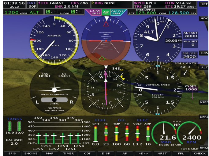
Analog Instruments: Standard analog 6-pack instrument display, including - analog HSI.
