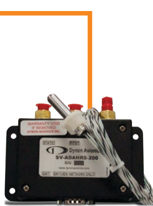
SV-ADAHRS-200 (Primary) Attitude & Pitot Static
